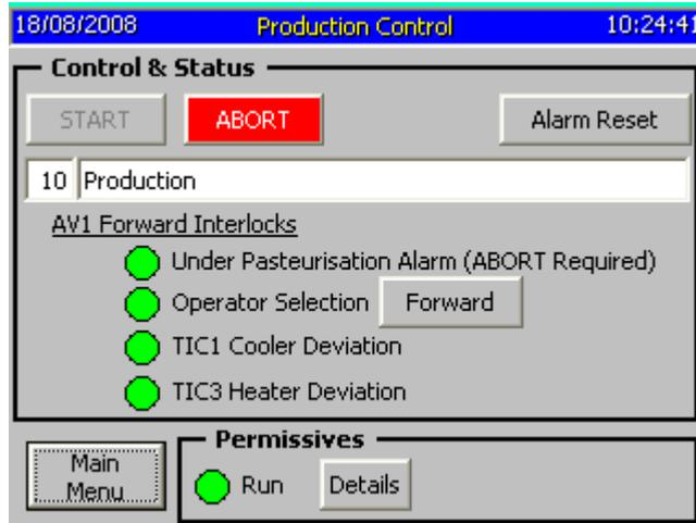
AV1 is deactivated to divert if any of the AV1 forward interlocks become true, this is indicated by a red lamp, as shown below.
